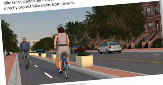
A street with a curb and plants-protected dual-lane cycle track.
