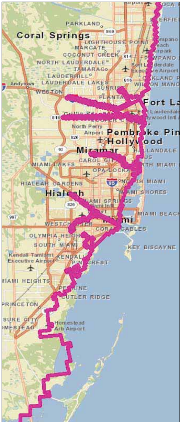
Figure 2.9 Interface between Inundated and Dry Cells - Hurricane Andrew
