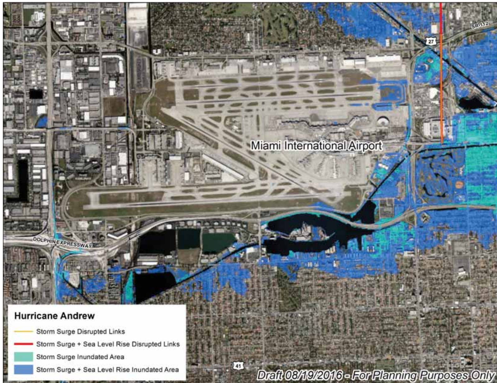
Figure 4.25 Hurricane Andrew's Impact on Miami International Airport
