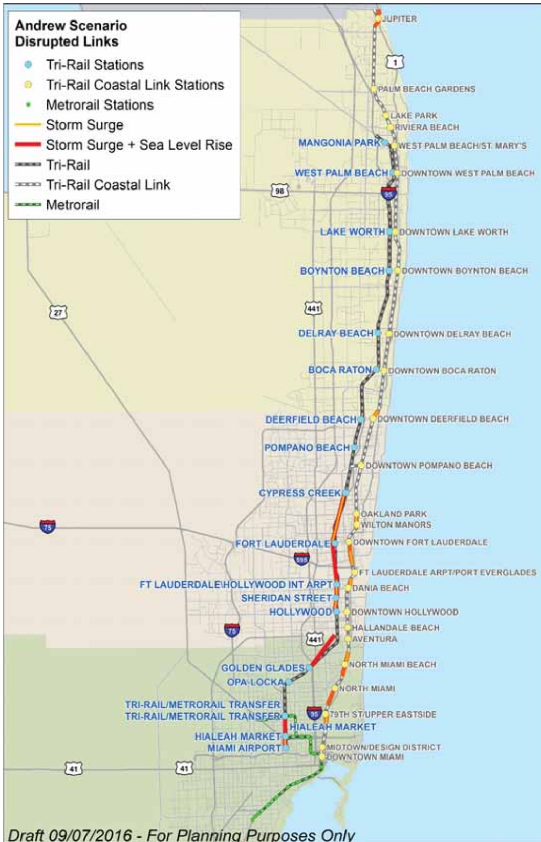
Figure 4.22 Hurricane Andrew's Impact on Tri-Rail and Metrorail
