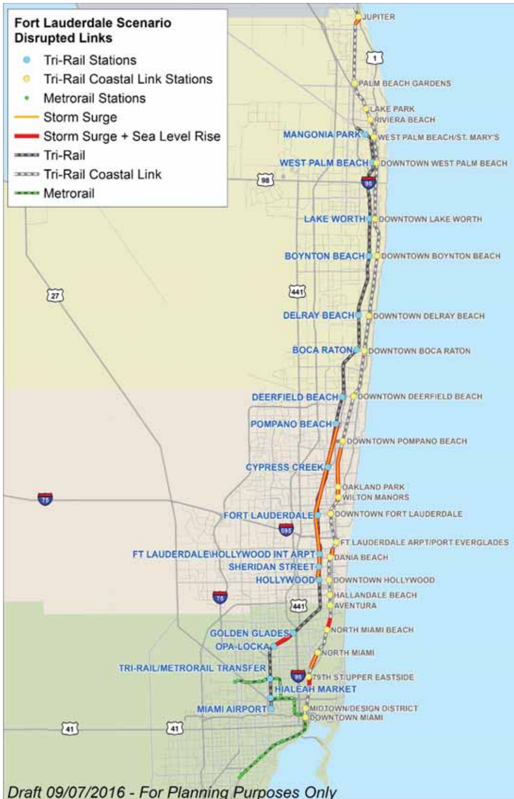
Figure 4.23 Fort Lauderdale Hurricane's Impact on Tri-Rail and Metrorail
