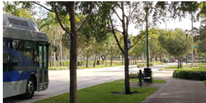
BCT Bus Stop on SW 84th Av. The bus bench faces away from roadway and ADA-compliant concrete pad is missing.
