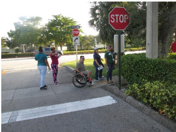
Many driveway exits require motorists to stop twice; once for the non-motorized users and then for motorists to enter the stream of traffic.
